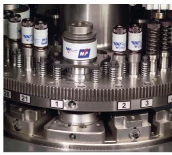
*A* 21-station turret configuration offers tremendous flexibility and capacity.
