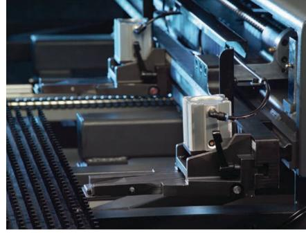
*Smart Clamp minimizes no-punch zones to reduce progressive move requirements and improve material utilization.*
