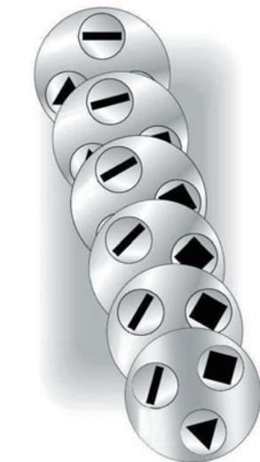
The Multi-Tool indexing mechanism allows any selected punch to be oriented in increments of 0,01° to any programmed angle automatically.
